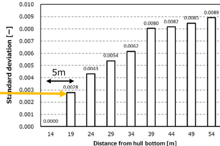
Standard deviation of overall average of relative flow velocity ratio at every layer to the shallowest layer
