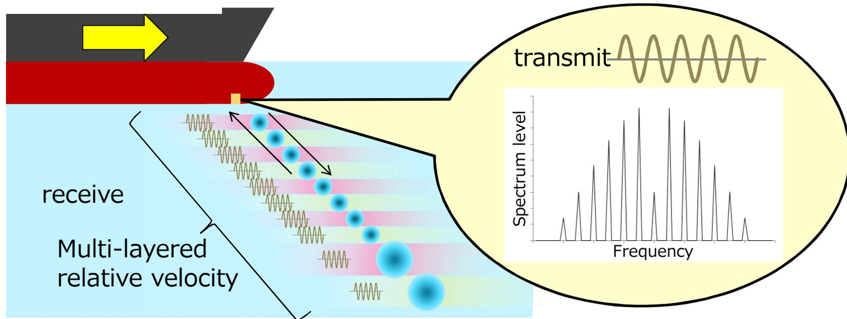
About N times amount of data can be obtained by measuring doppler shifts of each spectral peak at the same time independently. That means about N layers of relative velocity can be obtained.
