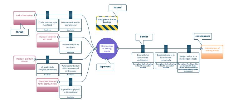
In order to determine effective monitoring points and preventive measures, it is also necessary to understand the causes of failures and their risk of occurring. Performing a Failure Mode Effect Analysis (FMEA) as part of the DCBM design process is recommended, to properly organise preventive measures and anomaly detection methods that can be used for the various identified failure modes and potential causes of malfunction for the components.
